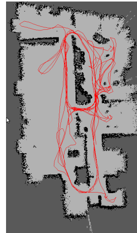
Figure 7: The robot path when selecting frontier points closest to the origin
