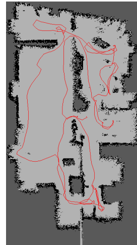
Figure 8: The robot path when selecting frontier points closest to the robot
